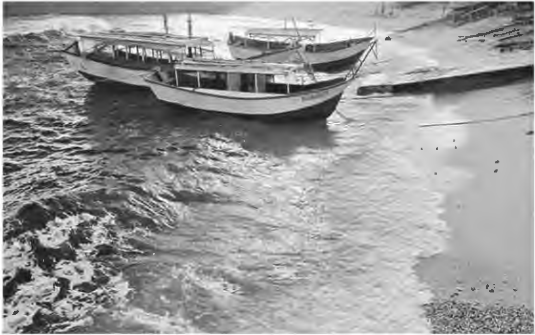
Figure 6. Local boats in Batanes province have rounded hulls, for better navigation in rough seas (Photo: Babiera, M; Source: Uy & Shaw; adapted from Hornedo, F., 2000; in UNISDR, 2008)
