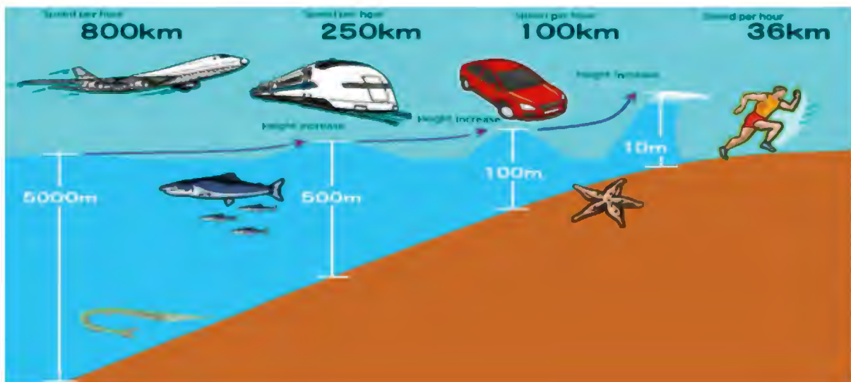
Figure 21. As tsunamis approach the shore, they become slower but the waves become higher. Tsunamis pack tremendous energy which can destroy buildings and other infrastructures (Figure: JMA)
