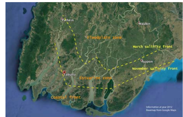
Figure 15a and b. Average salinity intrusion (1ppt line) in the Ayeyawady Delta and seasonal intrusion (adapted from Delta Alliance)
