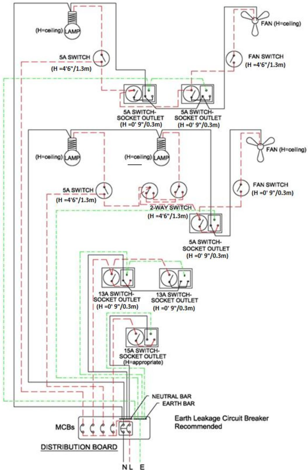
Figure 1: Wiring Diagram for a Typical Distribution Board Scheme in a Residential Building Flat
