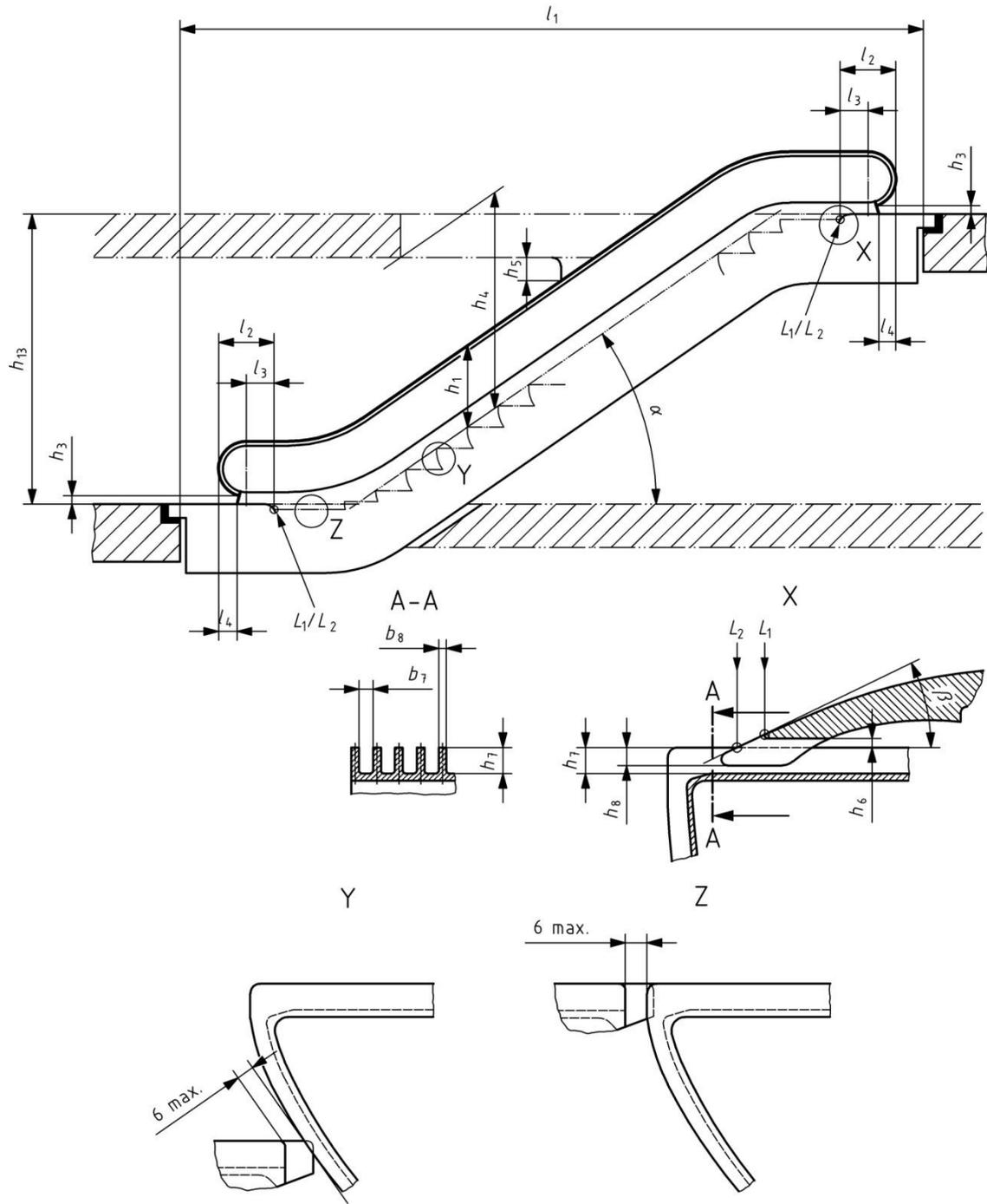
Figure 2 — Escalator (elevation), principal dimensions
